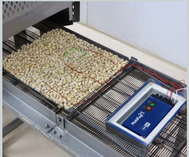
Testing in the MSU BSL-2 Pilot Plant includes validation of pathogen-reduction processes for nuts and other low-moisture food products.
