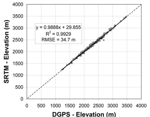
Fig. 2. Relationship between elevations obtained from a digital elevation model (DEM) acquired by the Shuttle Radar Topography Mission (SRTM) vs. their respective elevations obtained in the field (using a differentially corrected Global Positioning System receiver, DGPS). The root mean squared error (RMSE) was obtained using the 1-to-1 relationship (i.e., dotted line), while the  $R^2$  was obtained from the linear regression (i.e., continuous line).
