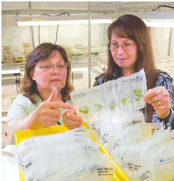
Hops plantlets can be stored in semipermeable plastic bags for 1 to 3 years without transfer but must be evaluated three times a year for viability. Technician Jeanine DeNoma (left) and plant physiologist Barbara Reed inspect plants stored with standard MS iron, which allows for longer storage than media with sequestrene iron.
