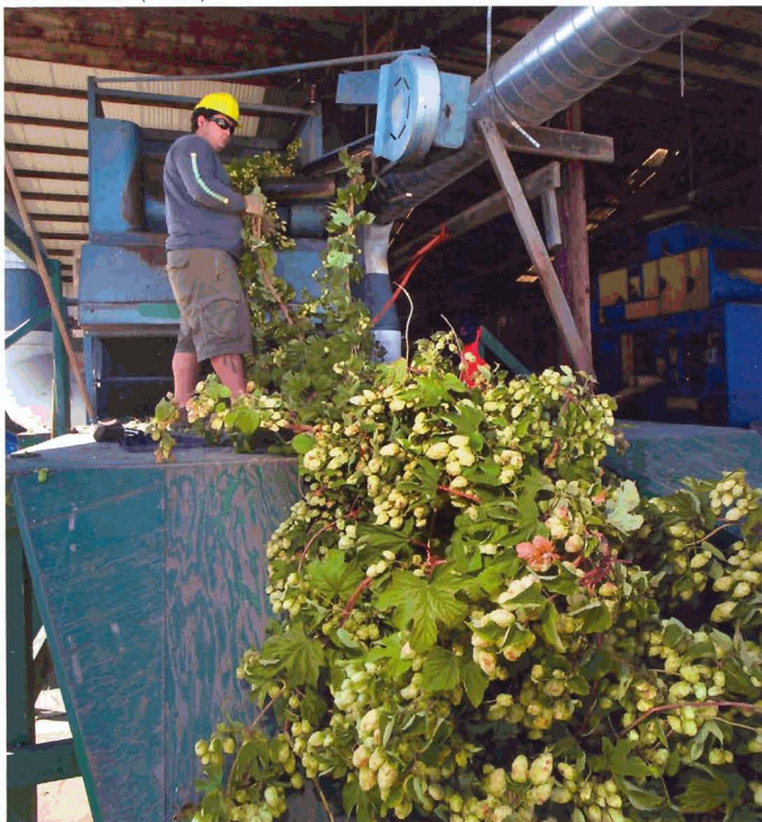
Oregon State University student technician Kris Judy loads recently harvested hop plants into the stationary picker for harvesting and separating hop cones from other plant material.
