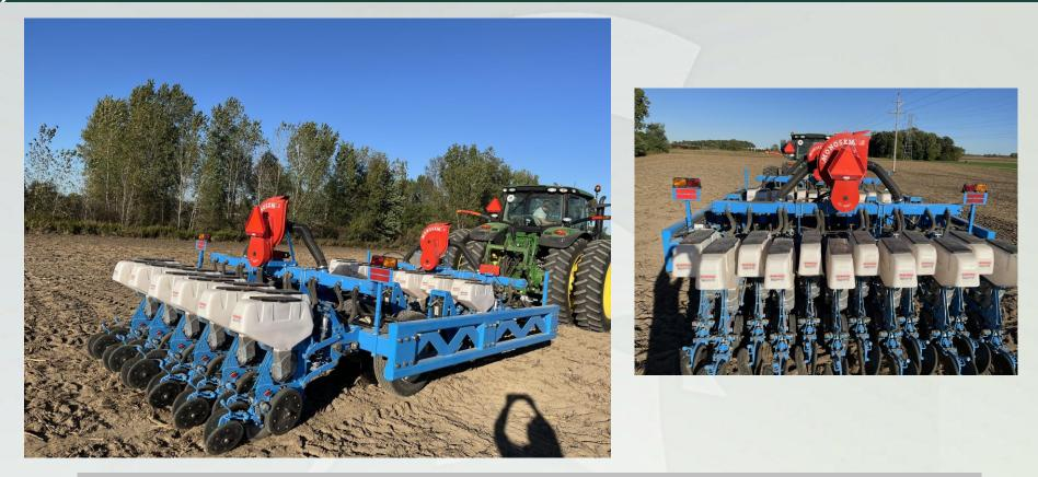
**Ongoing research**: New custom-build planter with capacity to plant in **5" row spacing** (using 2 toolbars, with row units spaced 10" apart on each)
