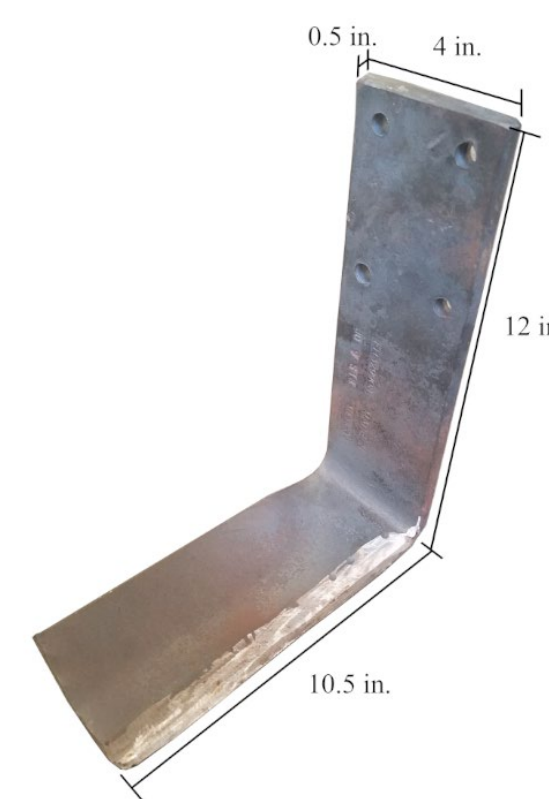
Figure 4. L-shaped blade with dimensions
