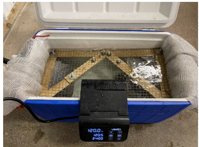
Figure 9. Hot water submersion using a sous vide mounted on a 30-gallon ice chest. Chestnuts placed in mesh plastic bags remained submerged by placing a wooden frame, fitted to the inside wall of the cooler, over the bags of nuts.
