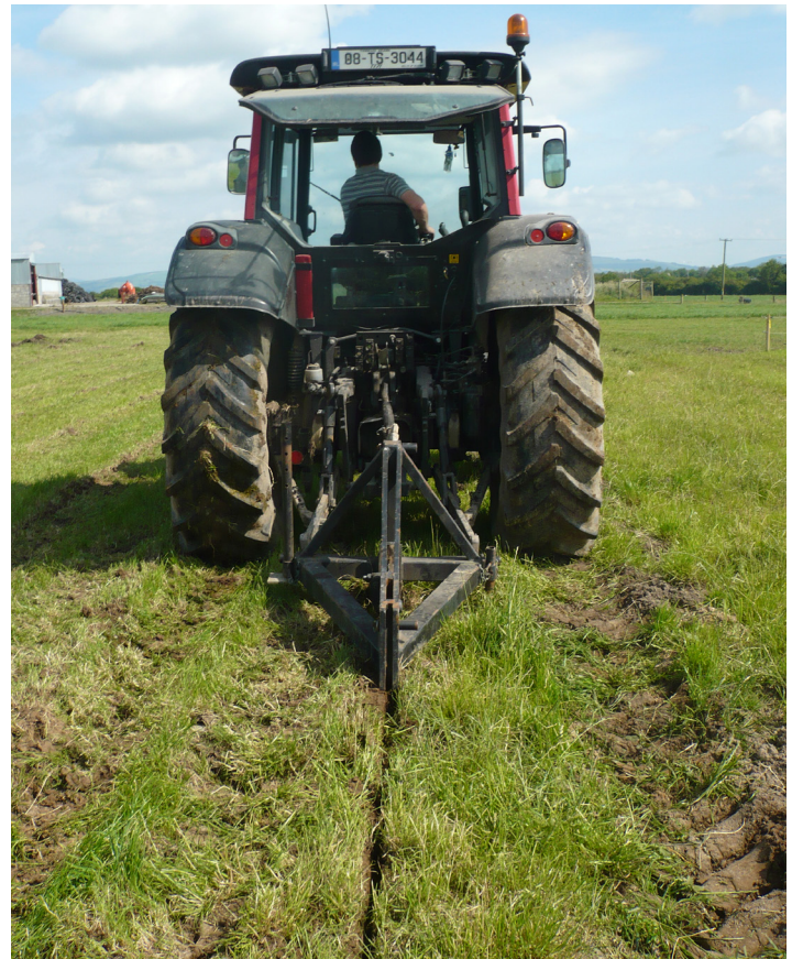
Figure 3- A tractor pulling a mole plow. The shank (leg) creates a blade-cut to break up the plow-pan and compacted surface layer to improve infiltration (Photo credit: Patrick Tuohy).
