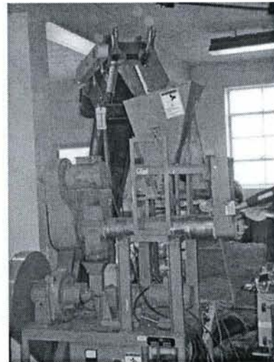
Figure 1. Picture of the pellet mill used to manufacture poultry litter and switchgrass pellets
