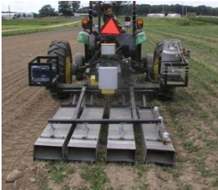
Figure 1. Configuration of the precision-guided shielded propane flame weeder. In the yellow box, a digital camera detects the crop row and allows for automated alignment of the entire machine in relation to the crop row. A 500,000 BTU liquid propane torch is mounted under each shield.
