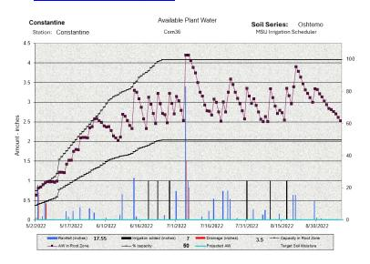
The MSU Excel Scheduler displays a graph of estimated available water in the root zone, making it easy to track for irrigation scheduling.
