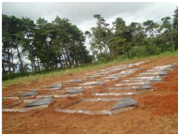
Figure 3. Lysimeters installed, in land with 6% slope, at Lichinga Agriculture Research Station.
