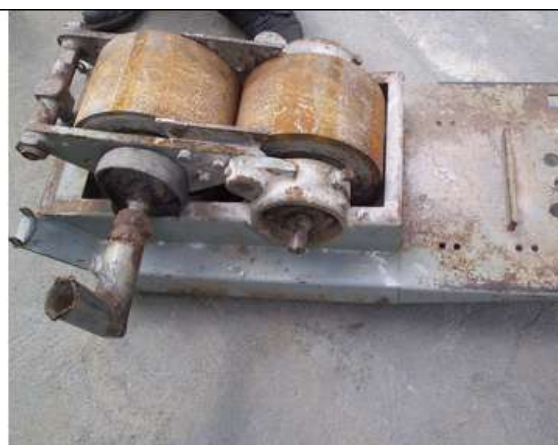
Fig. 5b. Manual grinder that is used to grind rock phosphate.
