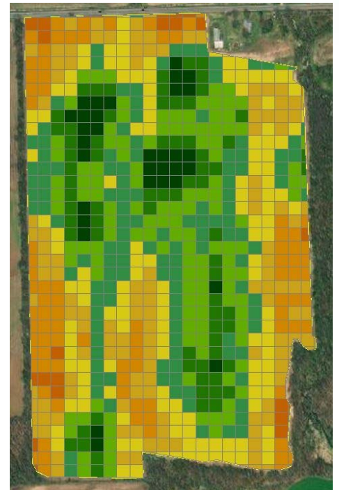
Figure 1 Normalized Difference Red Edge (NDRE) values at sidedress. Green areas indicate above-average biomass.
