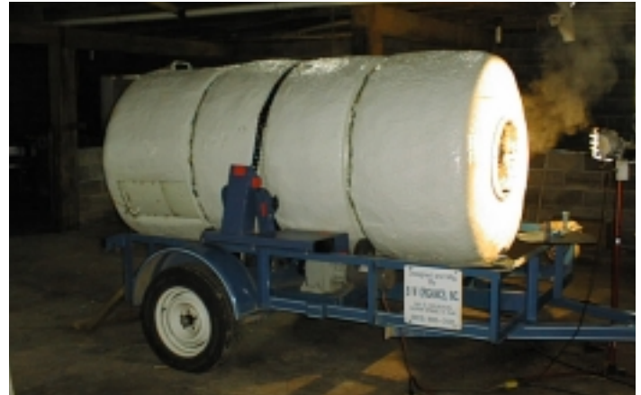
Figure 4. BW Organics Model 408 rotating drum in-vessel composter.
