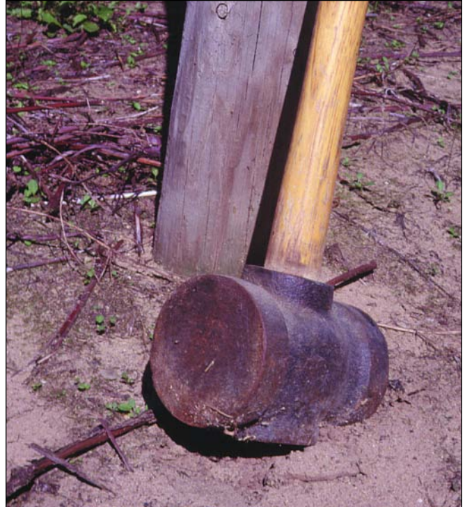
Fig. 26. This post maul has a head with a 3.5-inch diameter. It is used for installing or replacing a small number of posts.
