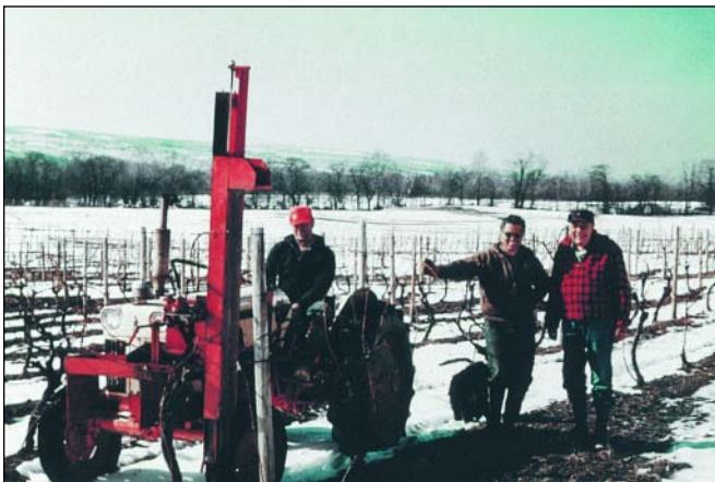
Fig. 25. Vineyard trellis posts are often installed with a hydraulic post pounder like the one shown here. (Stamp Farm, Rock Stream, N.Y.)
