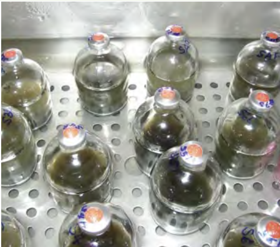
Once waste materials are “digested,” samples are bottled (above) and examined to determine their biogas methane potential.
