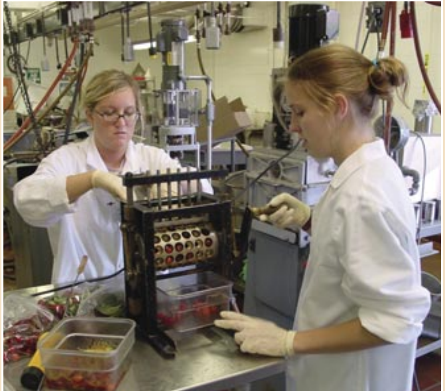
MSU biosystems and agricultural engineering undergraduate student Danielle Habitz (left) and food science master's student Claudia Place use a cherry-pitting machine to study the prevention of larvae infestation in fruit.
