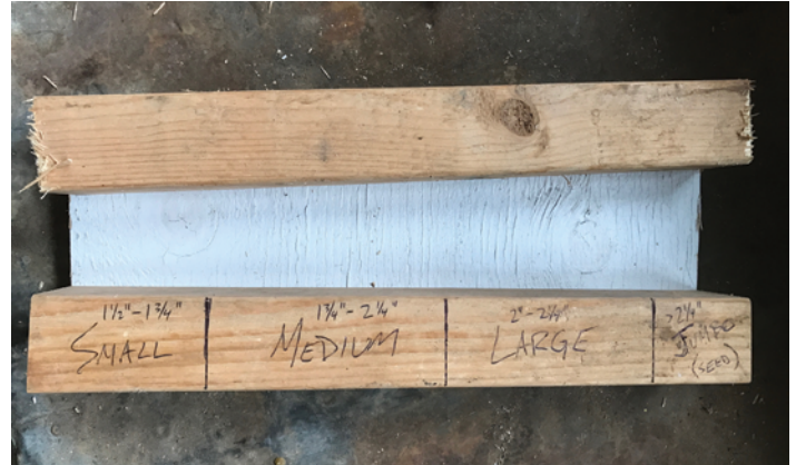
Simple tool used to grade garlic for sale. Garlic is passed between boards until head diameter is determined.
